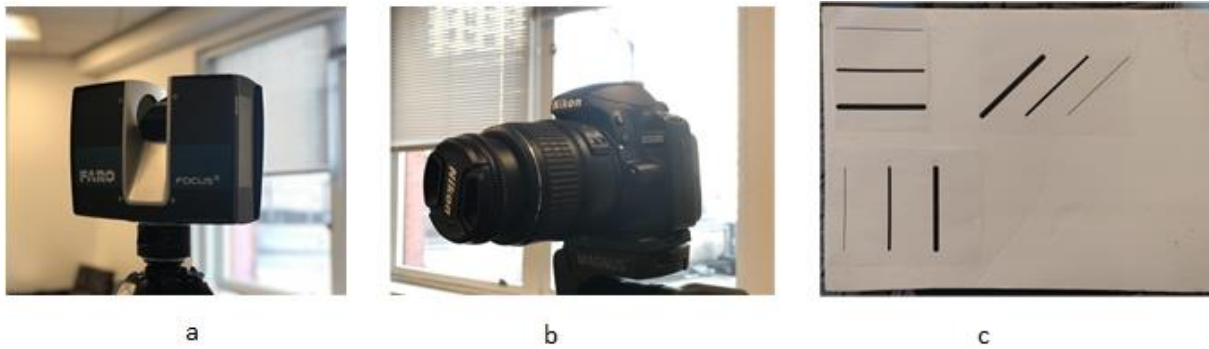
Figure 1. Experiment Setup. (a) FARO Focus S 150; (b) Nikon D3200; (c) Simulated cracks;
